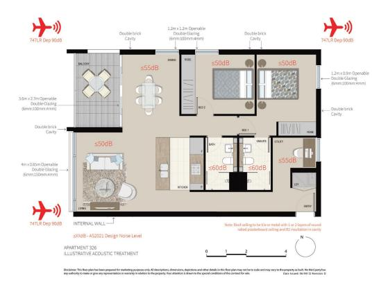
*Figure 7* - Indicative floor layout *Source: Turner Associates*
